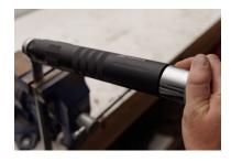
When assembly is completed the suppressor is ready to be used again. The AC338 should be maintained in this way each time after a range day if possible. If the AC338 is not at a minimum disassembled in the described way between range days, carbon deposits can build up on the interior surfaces of the suppressor and harden making disassembly progressively more difficult.
