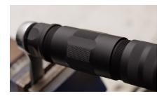
When unthreading the tube, it is common to see some particles and material in the threads. This is normal and can be cleaned with a small amount of a firearms solvent of your choice and a nylon brush.
