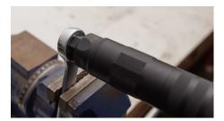
To disassemble the AC338, begin by securing the 1" socket and driver or wrench in a vice, as shown. This will serve as the holding point for the mount portion of the suppressor.
