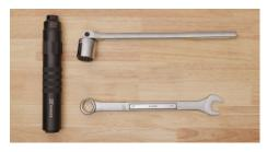
The tools required to assemble, disassemble, and maintain the AC338 are a 1" wrench or socket (mount) and 1 ¼" wrench or socket (tube).
