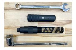
Once apart, the only things that you need to clean are the deposits off of the interior and exterior surfaces on the MonoKore™, and the interior surfaces of the tube. Use only firearms solvents, nylon brushes, and rags/towels. DO NOT USE METAL BRUSHES OF ANY KIND.
